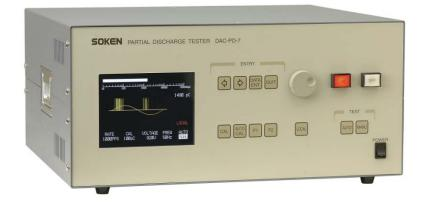
Partial Discharge measurement is non-destructive tests having higher detection sensitivity than withstanding or high resistance tests, and can be used to find insulation defects and early failures of solid insulations. DAC-PD-7 is ideal for quantitative diagnosis at production and inspection of electrical parts, such as EV motor, Photo-coupler, IGBT, and insulation materials etc.
