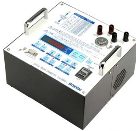
On Site Test Type: DAC-MRG-1
