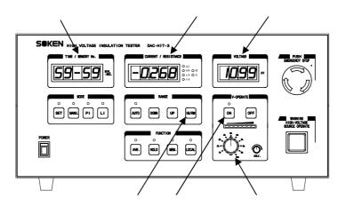
Measurement time, Memory No. Test voltage Test Voltage Applying Key Current and Resistance Current/Resistance switch key DC Voltage Change Switch
