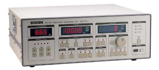
DAC-PD-3 provides Wide Band (10kHz~4MHz) and Narrow Band (10kHz~200kHz). Since bandwidth can be easily chosen according as the kind of test specimen and measuring sensitivity, etc., DAC-PD-3 is available with partial discharge tests such as electric equipments, electronic parts and insulating materials.
