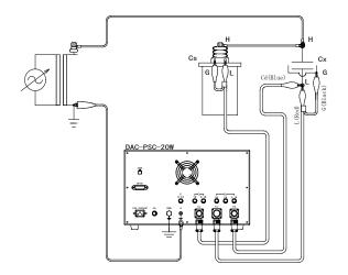
■Connection with Expanding CT (When CT is ON)
